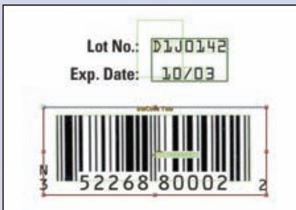
Typical Pharmaceutical Application for Date Lot Code and Barcode Match String Verification
